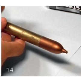
Depending on the result to achieve, we polish in some way or another, less polishing would mean an older metal while polishing a lot means newer metal.
