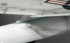
Make sure the streaking run in the direction of airflow.
